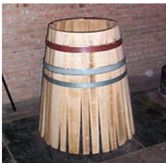
Image 10: Image of shaped staves being assembled into a water-tight barrel.
